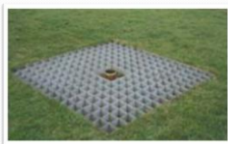
Gauges can be designed to minimise errors from splash
