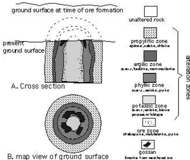
Figure 3. Schematic cross section (A) and map view (B) of a porphyry copper deposit, illustrating that the hydrothermal envelop makes a larger target for exploration (after Lowell and Guilbert, 1970).
