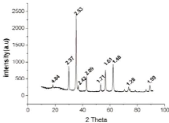
Fig. 1: X-ray diffraction of MNPs.
