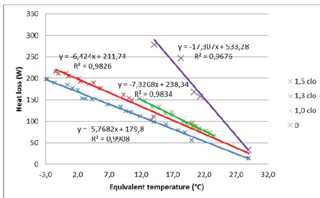
Fig. 3: Heat loss of humans as a function of the equivalent temperature in different clothes.
