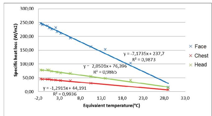
Fig. 4: The specific heat loss of the face, chest and head when 1.3 clo clothing covers the body.
