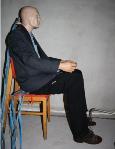
Fig. 1: Thermal manikin in a seated position.
