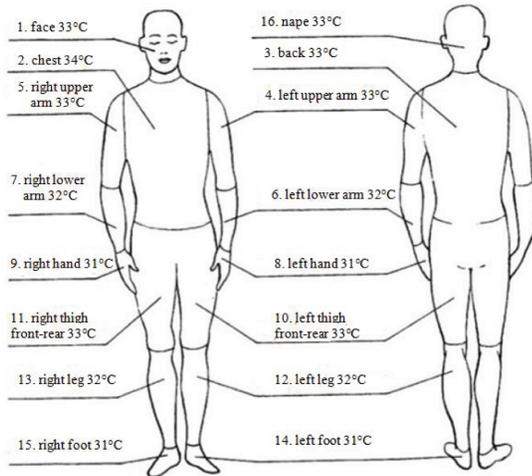
Fig. 2: Surface temperature of different parts of a thermal manikin.
