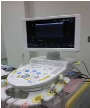
Figure: Hitachi (EZU-MT30-SI HI Vision Avius, Hitachi, Japan) US units equipped with a linear probe of a frequency 10 MHz.
