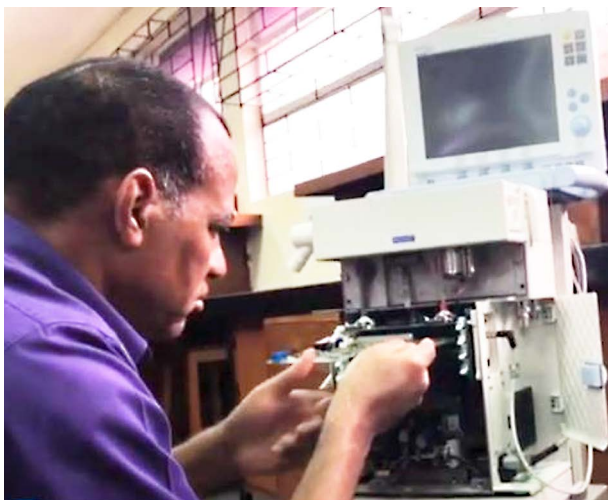
Staff at the Faculty of Engineering repairing ventilators
