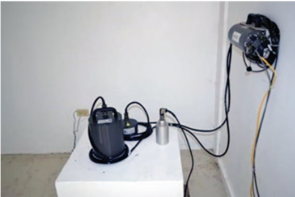
Figure 2. Equipment at one of the upgraded seismograph station at Stony Hill.
