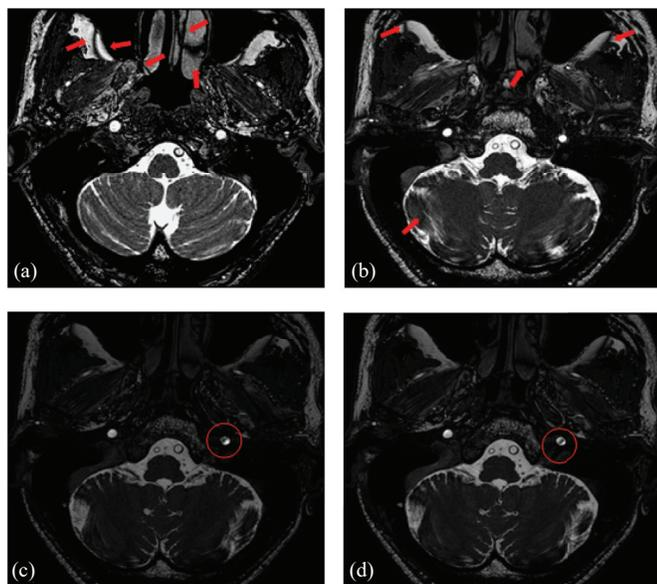
Fig. 4: Magnetic field inhomogeneities at different locations within field of view. (a)(b) Unpredictable imaging artifact in the form of banding has appeared in the image (arrows); (c)(d) and blood vessel signal loss (red circle) has also occurred.
