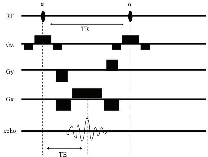
Fig. 3: Balanced fast field echo pulse sequence diagram. Balanced fast field echo has a fully-balanced gradient waveform, permits the magnetic moment to achieve a steady state and has inherently automatic flow compensation. Abbreviations: RF = radiofrequency, Gz = slice selection gradient, Gy = phase encoding gradient, Gx = frequency encoding gradient.
