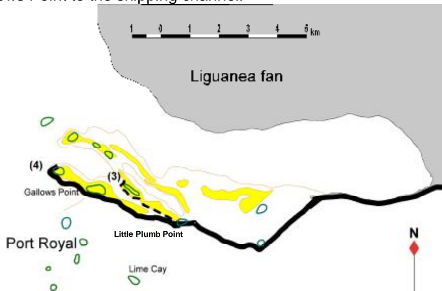
Figure 7. Later, longshore drift extended a spit (4) from Little Plumb Point past what is now Gallows Point to the edge of the deep channel. Black line, spit; green, cays; yellow, shoals; peach line, extent of shallow water.
